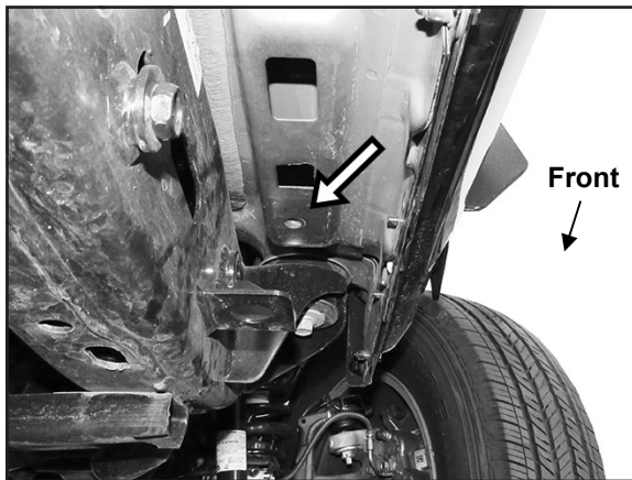
(Figure 5) Locate threaded hole in floor (arrow) at passenger/right front mounting location.
